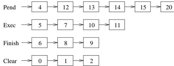
Figure 11: Central queue data structure (with cancelled/failed and restarted epochs).
