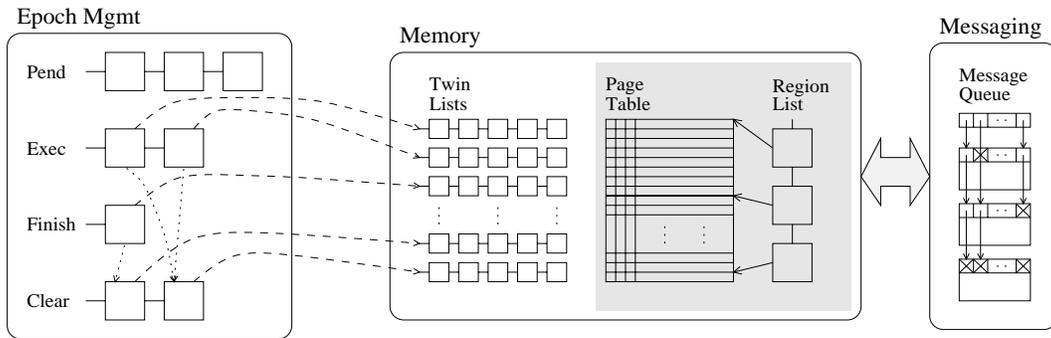
Figure 10: High-level view of software-only implementation. Shaded structures are *not* located in shared memory. The messaging subsystem is used to broadcast necessary updates, as well as during initialization (and for any other exchange of information that do not fit in central epoch queues and linked structures).
