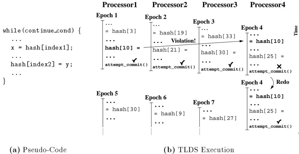
Figure 8: Example of TLDS execution.
