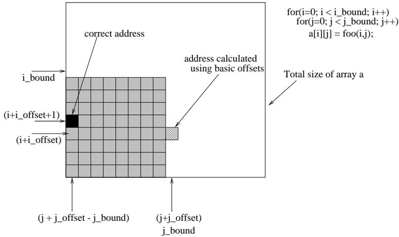
Figure 7: Computing the correct prefetch address with multi-dimensional software pipelining.
