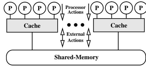
Figure 14: Base architecture for the TLDS coherence scheme.
