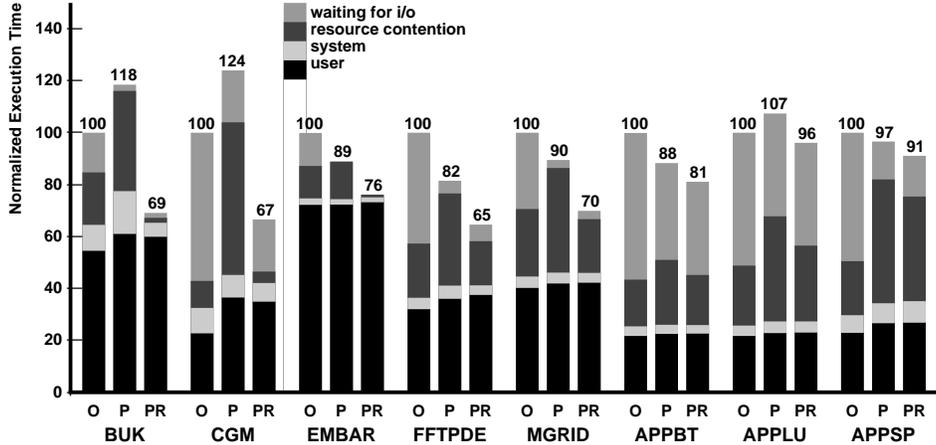
Figure 5: Impact of prefetching and releasing on the execution times of the out-of-core applications. (O = original; P = with prefetching only; PR = with prefetching and releasing.)
