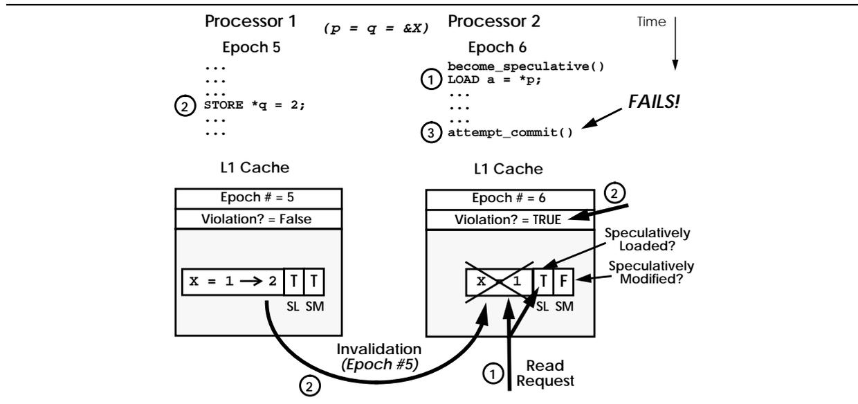
Figure 13: Using cache coherence to detect a RAW dependence violation.
