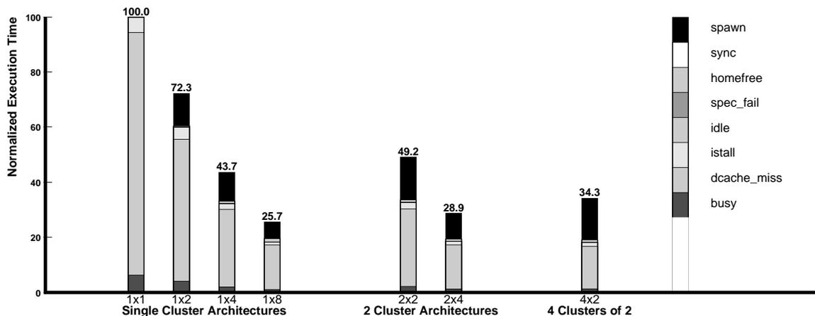
Figure 16: Region performance of **buk** on a variety of cluster architectures ( $N \times M$  means  $N$  clusters of  $M$  processors).
