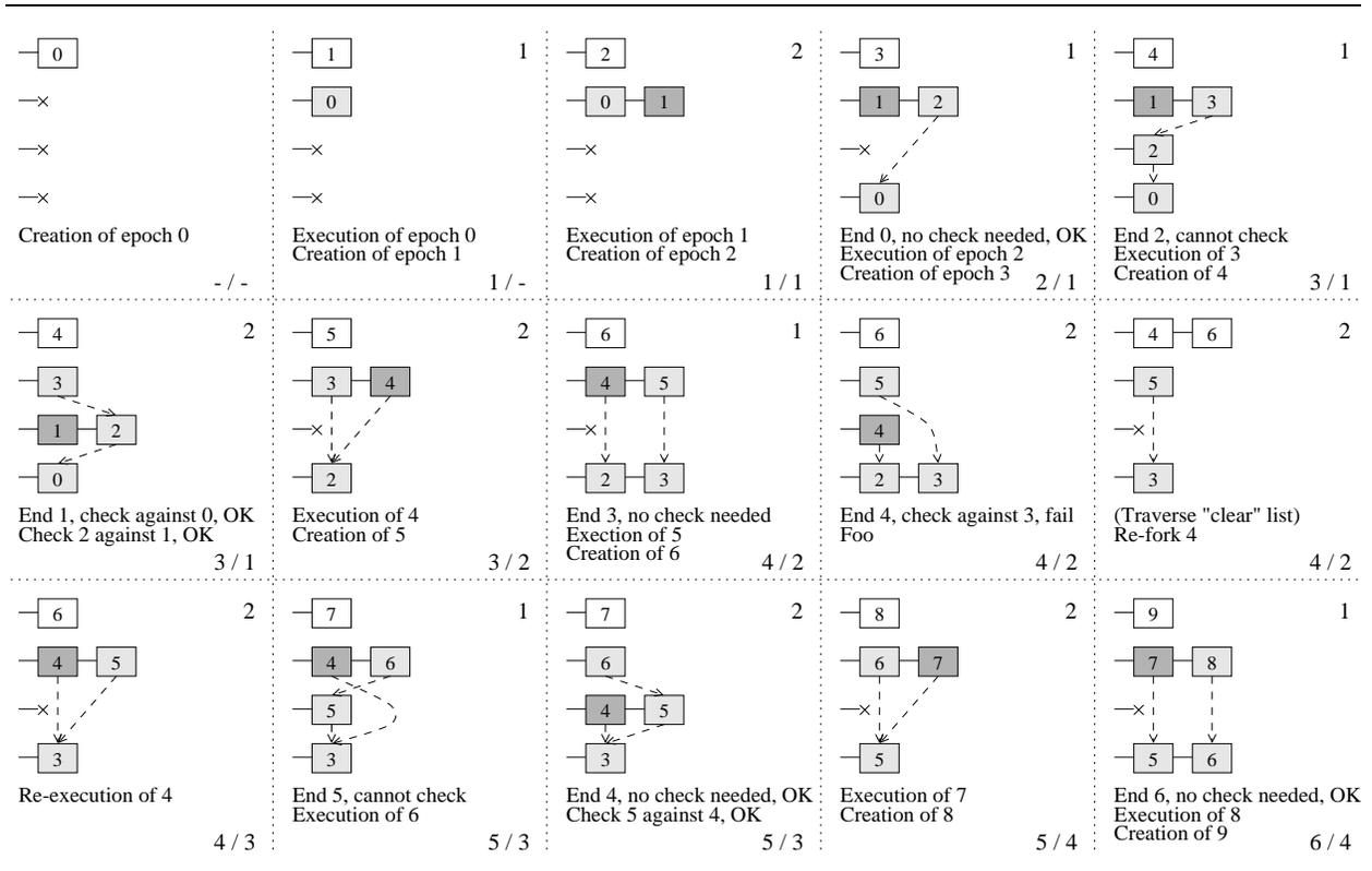
Figure 12: Central data structure during progress of execution, on a system with two processors. The “last seen” pointer is shown with a dashed line. The iteration number of the main loop for each processor is shown at the bottom right of each picture. The processor performing the actions listed in each picture is shown on the top right. Epochs executed on the first processor are lightly shaded, whereas epochs executed on the second processor are shaded dark.
