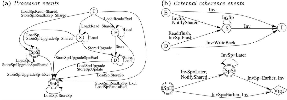
Figure 15: Baseline coherence scheme for speculation
