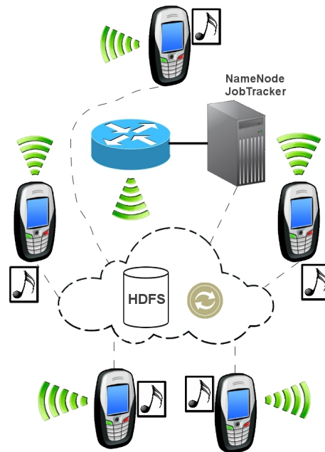
Figure 6.1: Overview of design of MusicDJ . Each mobile device contains its own music files on its own local filesystem
