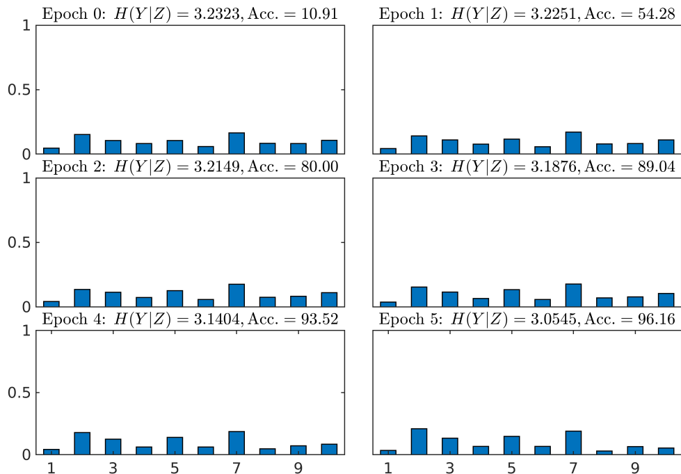
Figure 5.18: Layer 1 of a 3-layer MLP. The class distributions of the selections of two features over the first five epochs, the corresponding feature-wise conditional entropies, H(Y|Z) , and the total classification accuracy of the model at that epoch. Epoch 0 refers to the state prior to training (i.e. the random initialization).
