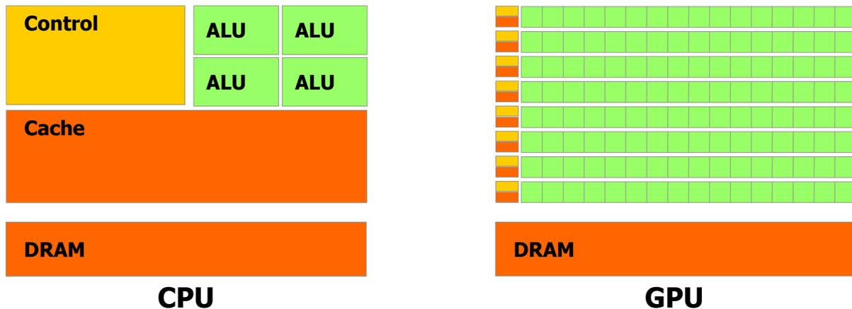
Figure 1.1: The GPU has more transistors devoted to data processing
