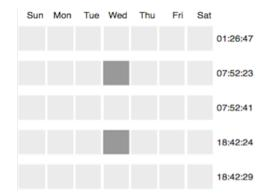
Figure 4-5. A short-term view of medication taking data for one day. Each row represents the state of the pillbox doors. A darker shaded door indicates it is opened. This shows the user taking her morning pill at 7:52am and taking her evening pill at 6:42pm.
