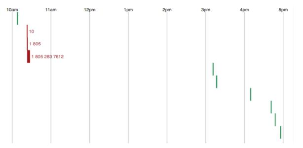
Figure 5-3. Detailed, short-term view of phone calls on a particular day, showing how the user at approximately 10:25am misdialed twice and successfully dialed the number on the third attempt. The horizontal width of the bars represents the length of the call. A bar is marked in red if it is part of an episode of misdialing. A green bar represents either a correctly dialed number or an incoming call if no number is displayed next to it.
