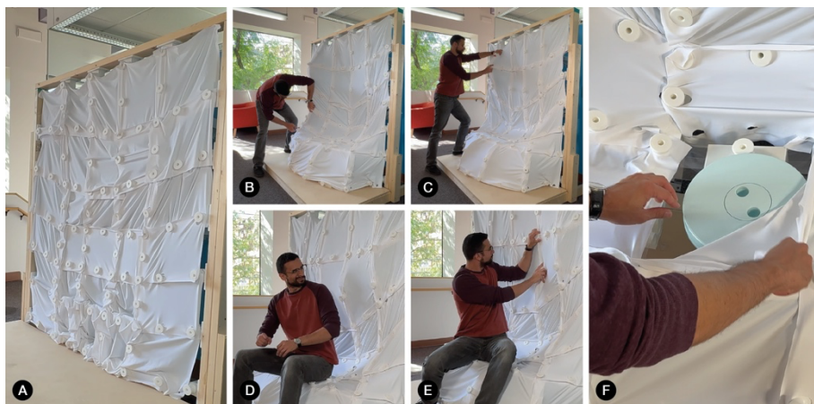
Figure 5. In its default state, our sculptable mesh surface is a flat plane (a). A person can pull on the edges and vertices to create forms such as a bench (b,c). They can use physical items, such as a stool (f) to interact with their creations. In this example, a person notices that their sculpted bench is uncomfortable (d), and so they make a modification (e).
