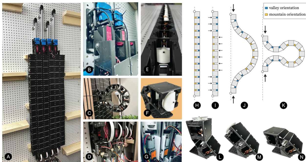
Figure 7. Our robotic surface consists of four fully-actuated columns, flanked by two decorative columns (a). Each column contains seventeen double-hinged cells, which can be constrained in either a valley (l), rigid (m), or mountain (n) orientation. These constraints are achieved by rotating a plastic clamp with a low-cost servo motor (e,f). For each cell pair, the clamp prevents either one or both sets of hinges from opening. After configuration, a belt-drive system (g) squeezes the column endpoints together, resulting in a rendered shape (c). This process is illustrated in (h-k), which models unconstrained hinges as fixed-length tendons, and models constrained hinges as ultra-stiff springs. The first and last cells are attached to servo motors (b,d), used for deployment and retraction procedures. All electronics within the column draw power from a shared 6V bus, running on flexible cables that are integrated into the cell structure. However, the servo motors attached to the topmost cell (b) are powered by a 7.4V rechargeable battery, to compensate for a small voltage drop across the column.
