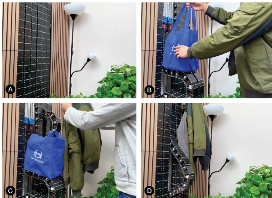
Figure 1. An interaction with a room-scale robotic surface (specifically, the robotic wall in Chapter 5). In the default state (a), the surface is flat, embedded in the wall. When a human approaches with a grocery bag, the surface morphs into a shelf (b) and a coat hook (c). When the human takes the bag and leaves, the shelf folds back into the wall (d).
