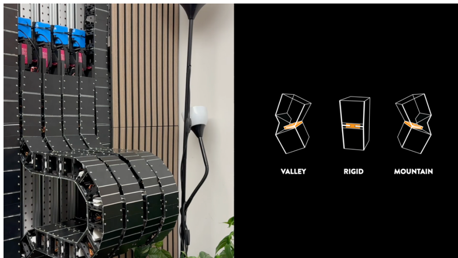
Figure 7. A shape-changing robotic wall (left) composed of multiple reconfigurable columns. Each joint can be clamped in either a valley orientation, rigid orientation, or mountain orientation (right). Then, when edges are squeezed from the surface, shapes pop out of the plane.
