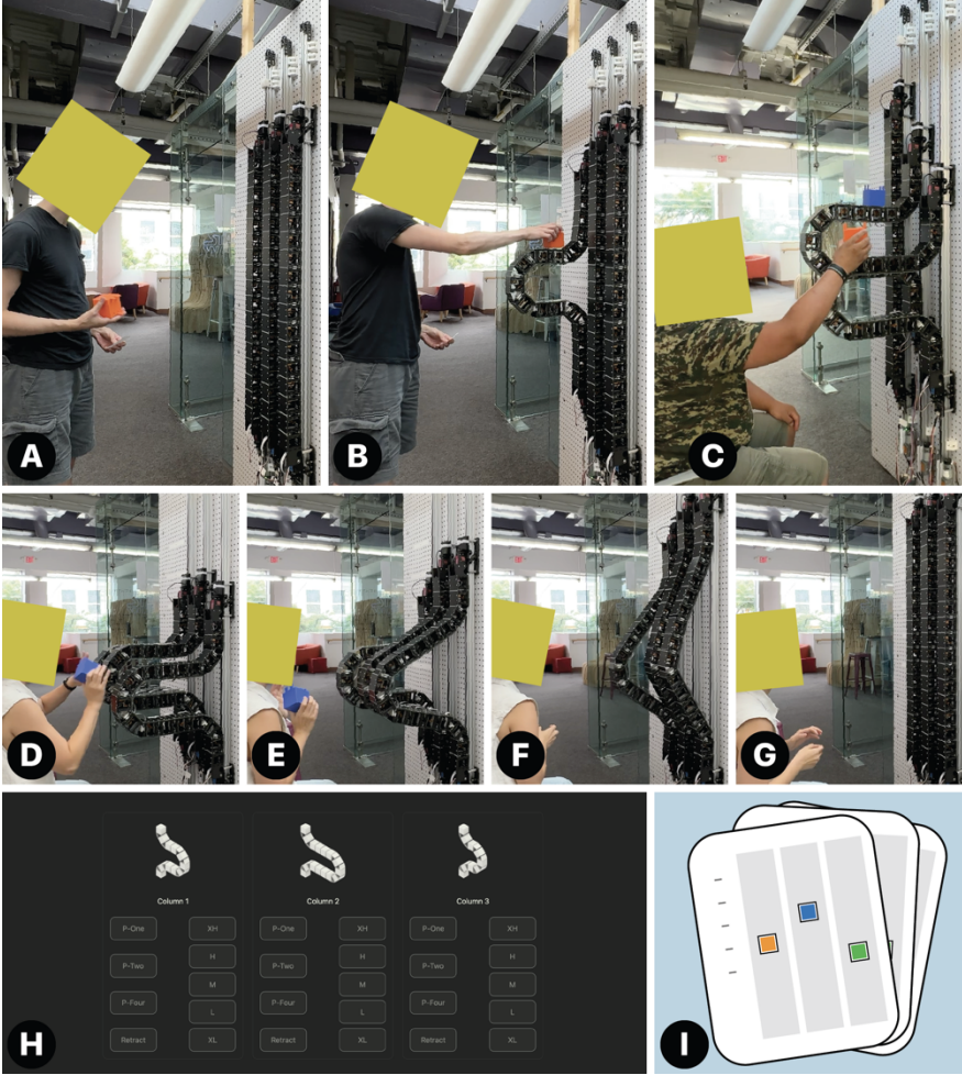
Figure 8. In our Wizard-of-Oz elicitation study, participants interacted with our shape-changing robotic wall. They were given a series of cards (i) and tasked with placing colored blocks on shelves at varying heights. Participants had to solicit shelves from the wall, both while standing (a, b) and sitting (c). After placing all blocks, and adjusting the heights of the shelves, they had to return the wall to the flat state (d-g). The robotic wall was controlled by human operator, using a graphical interface (h).
