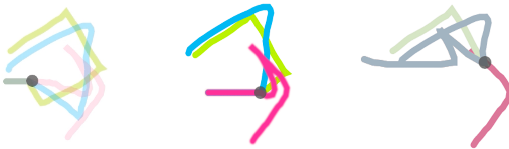
Figure 9.2 Example of Octopocus-inspired feedback technique of overlaying multiple alternate interpretations using opacity (left), blur (middle) and saturation (right) to reflect probability. The dot is the location of the touch position. The user is drawing an arrow pointing right.
