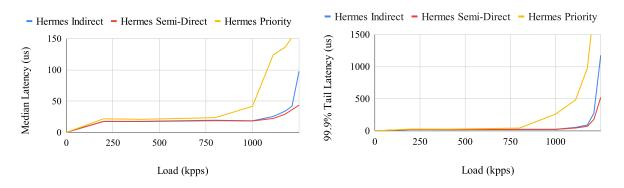
Figure 6: Load vs Median Latency (left) and 99.9% Latency (right)
