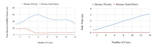
Figure 17: Components of SoftIRQ Process Time: Time between SoftIRQ Checks (us) and Uthread Parking Time (us)
