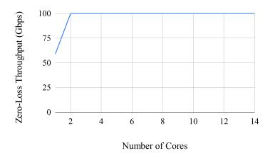
Figure 18: Throughput Scalability: Zero-Loss Throughput vs. Number of Cores
