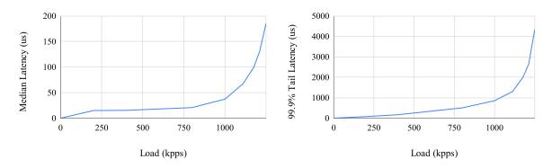
Figure 8: Hermes Indirect: Load vs Median Latency (left) and 99.9% Latency (right)
