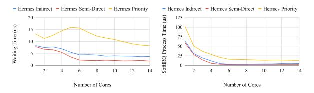
Figure 16: Components of Time to Uthreads: Waiting Time (left) and SoftIRQ Process Time (right)
