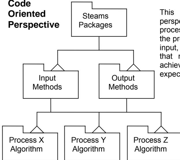
This view represents a code oriented perspective of the system showing three processes the essential elements that make up the processes. Common packages for streams, input, and output inherited by the packages that make up the process algorithms help achieve the expected interchangeability expected by the stakeholders
