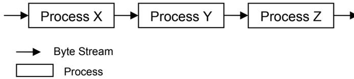
This view represents a runtime perspective of the system showing three processes X, Y, and Z. Assume that the user expects processes to be easily interchanged and/or replaced with new processes.
