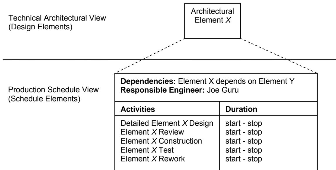
This illustration shows how each element of the architecture is decomposed into schedule elements. Each element then is rolled up to create a system production estimate.
