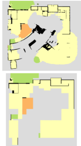
Figure 7.2: Using the model to segment the Majlis Area of CMUQ. Left: PNG image, Top: Room and wall segmentation by model, Bottom: Room and wall segmentation after post-processing
