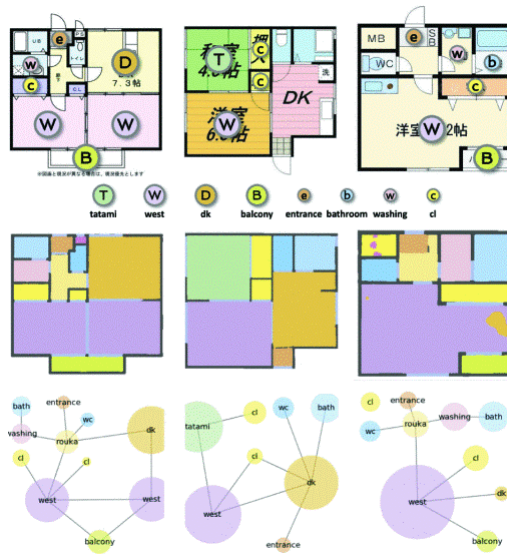
Figure 3.4: The process of taking a PNG image of an indoor space, segmenting it and extracting the graph [24]
