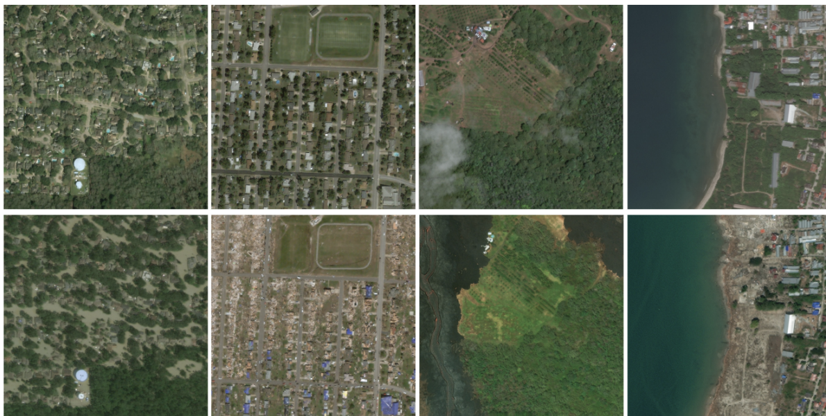
Figure 2.1: Example paired images from xBD dataset [6]. Pre-disaster imagery (top) and post-disaster imagery (bottom) for Hurricane Harvey, Joplin tornado, Lower Puna volcanic eruption, and Sunda Strait tsunami
