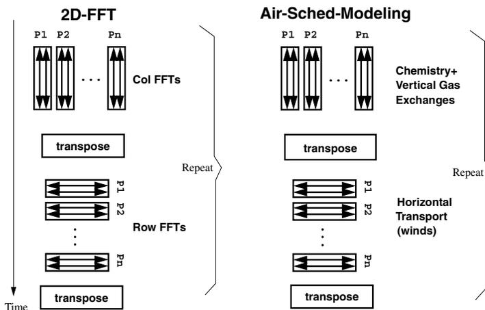
Figure 5.2: Block diagram of two application kernels showing their natural decomposition into compute and communication phases. 2D-FFT (left) and Air-shed modeling (right).
