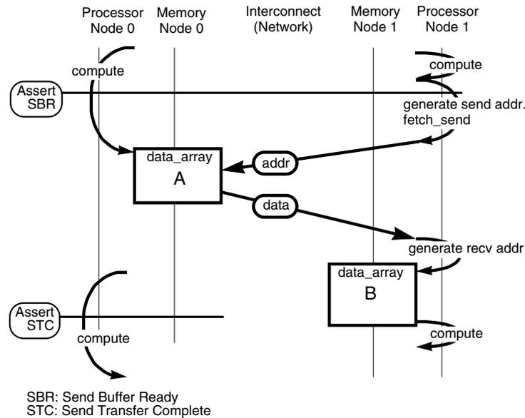
Figure 4.9: Control requirements and assertions in the of the fetch model.
