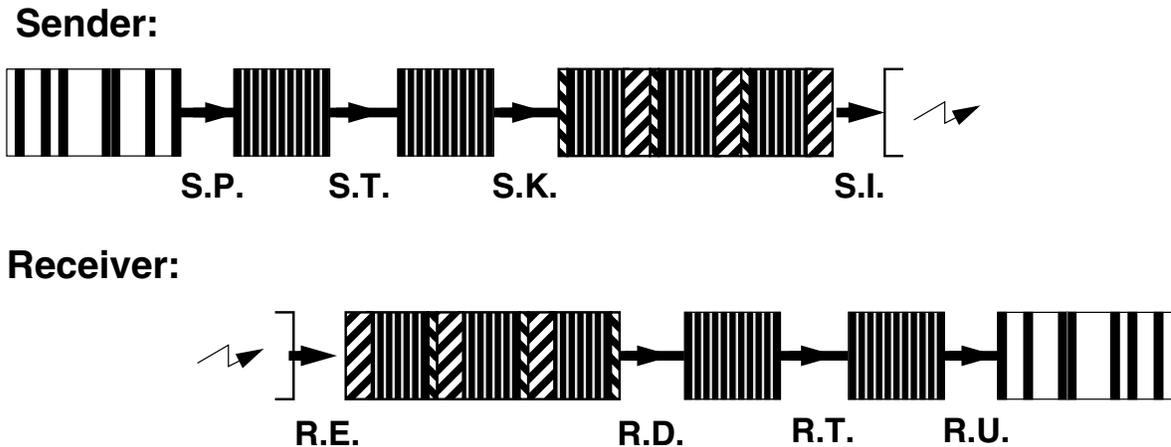
Figure 5.1: Potential copies of data elements as they occur in traditional message passing (e.g. PVM) due to coalescing of non-contiguous data transfers, protection domain crossing, and buffering to comply with synchronization semantics of postal model.
