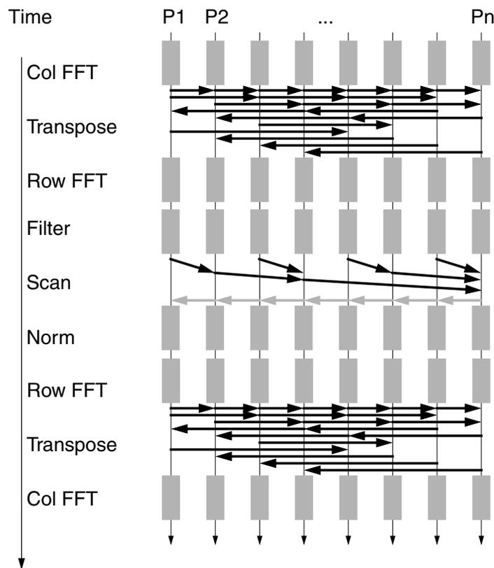
Figure 5.3: Computation and communications phases in typical applications.
