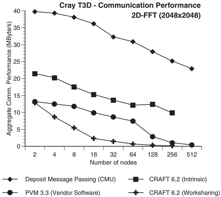
Figure 7.3: Per processor communication performance of a 2048 × 2048 point 2D-FFT for different machine sizes of Cray T3D.
