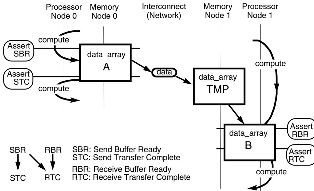
Figure 4.7: Control requirements and assertions in the of the postal model.
