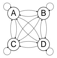
Figure 4: Four-state Markov model alphabetcomprised of four symbols. Letters indicate states; arrows indicate transition probabilities. A transition can be made from any state to any other state, with a given probability.
