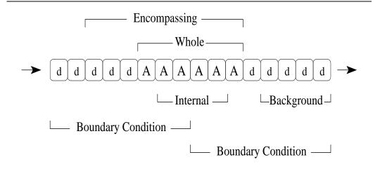
Figure 1: The ken of an anomaly detector: different views of an anomaly (depicted by AAAAA) embedded in a sensor-data stream (depicted by ddddd) from the perspective of a sliding-window anomaly detector. Arrows indicate direction of data flow.
