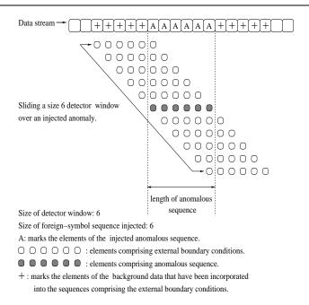
Figure 3: Foreign-symbol-sequence anomaly injected into background data. External boundary conditions are shown for detector window size of 6 and anomaly size of 6: DW = AS.
