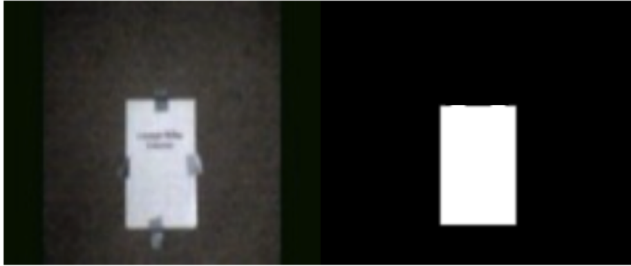
Figure 2.3: Binary mask (right) created by thresholding pixels in image (left)
