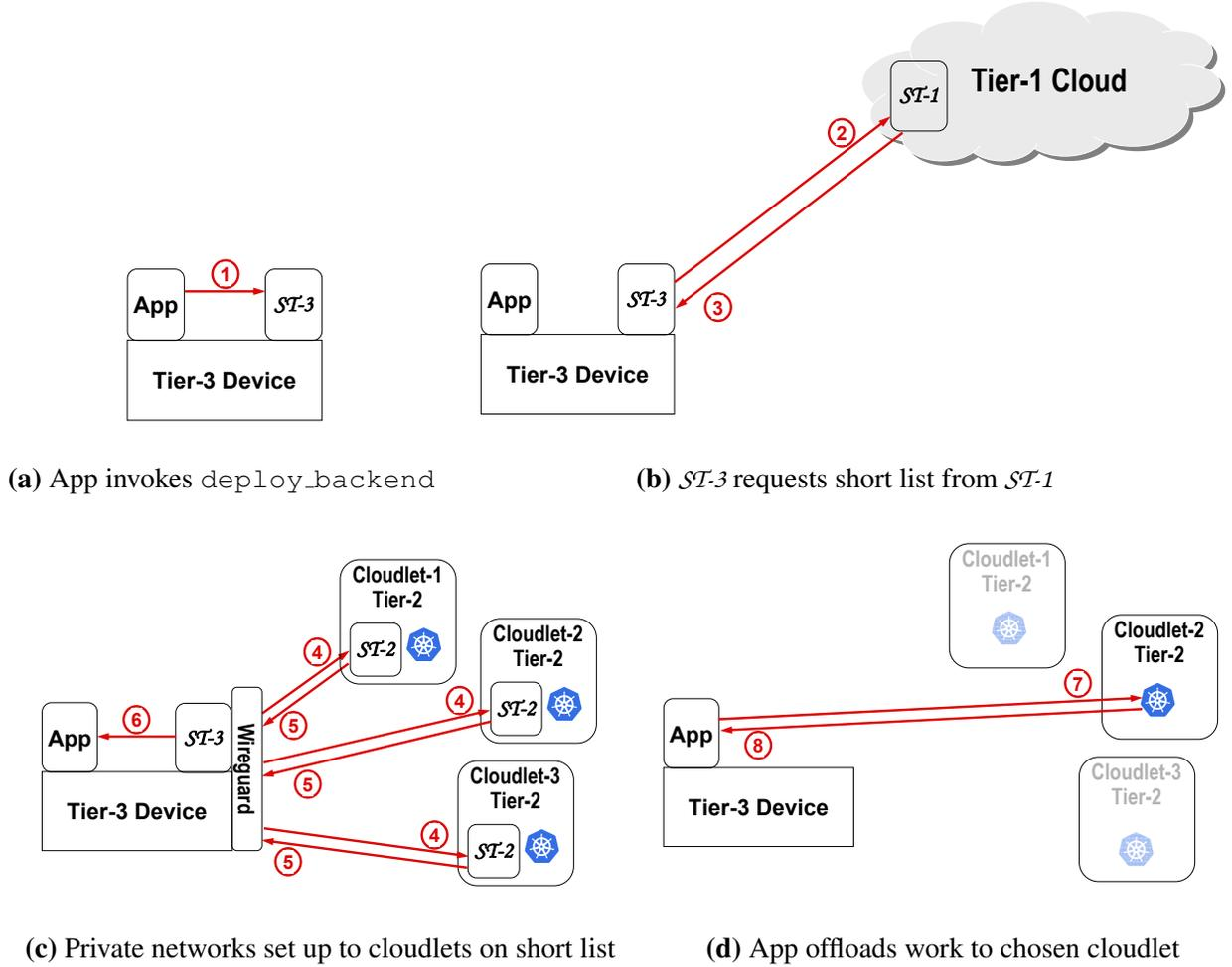
**Figure 4: Cross-Tier Workflow of Cloudlet Discovery and Association**
