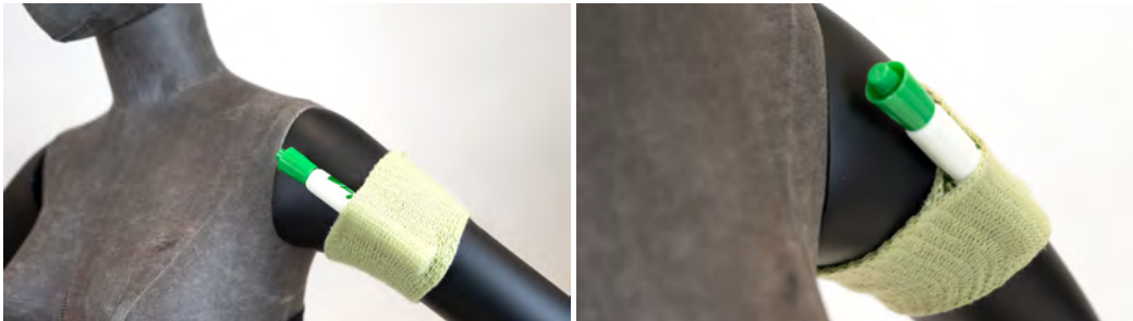
Figure 13.10 To produce open pockets such as these, the knitter must switch the carriage cam settings every other row, and the rack setting every row. The system helps the knitter keep track of these.
