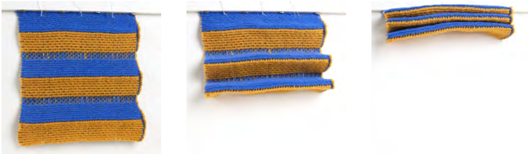
Figure 5.11 Hinge areas allow the active position of a sheet-shaped sample to fold along pleat lines.
