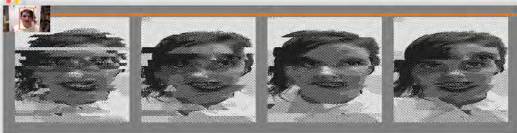
Figure 10.5 A screenshot of the view the weaver could see during the weaving process, with a small live video feed showing the portrait crop area and a preview of the woven structure in progress. The aspect ratio of the image is distorted to account for the non-square “pixels” of woven interlacement, which vary according to relative warp/weft thickness and other factors.
