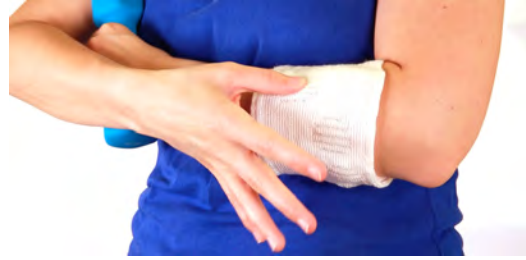
Figure 6.16 A soft control pad. Different thickness provide tactile cues to the location of capacitive button traces.
