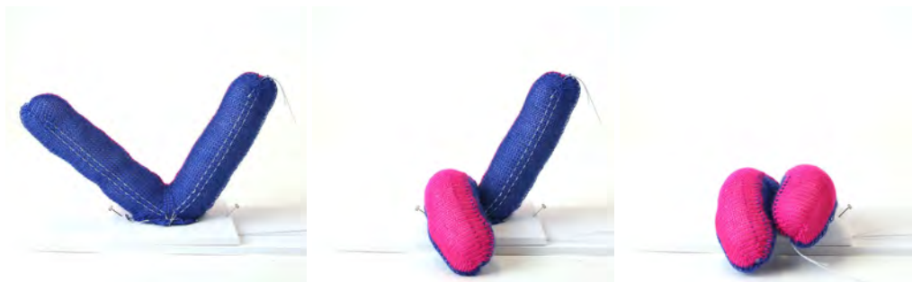
Figure 5.13 A horizontal tube with inlaid tendon and decrease shaping to bend the tube into a v-shape.
