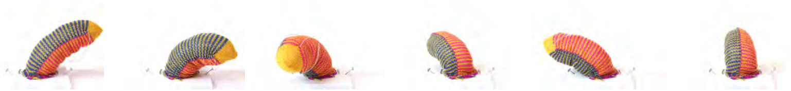
Figure 5.18 The three-way tentacle combines vertical tendon and shaping techniques: it has three vertical tendons and is shaped with decreases at the top.
