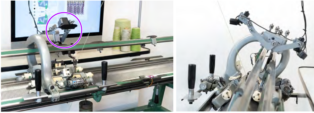
Figure 13.6 A pair of webcams is mounted to the “bow” that connects the front bed and back bed carriages. Each camera is positioned to capture the switch positions for its carriage
