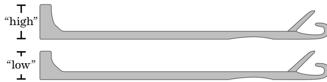
Figure 13.3 “High” and “low” needles differ only in the height of the selector tab, which is the part that protrudes out of the needle bed to be caught by the carriage cams.
