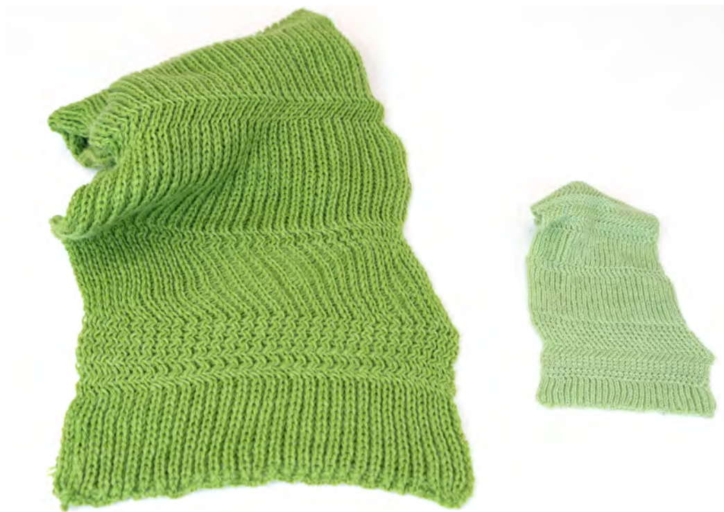
Figure 13.8 Because I track the machine operations, I can “replay” them on any Knitout-compatible machine. In this case, I have knit a duplicate scarf on a Shima Seiki SWG091N2, which has a much smaller stitch size than the Dubied.
