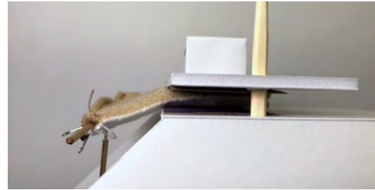
Figure 6.8 For stiffness testing, each swatch was lightly clamped to its center line between two sandpaper surfaces. The free edge was successively loaded until it bent below a 45° reference line.
