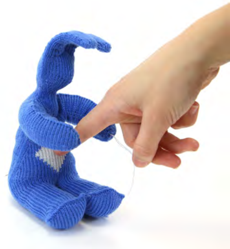
Figure 5.20 The bunny combines both tube types, both tendon types, both shaping techniques, and sensing. It is formed similarly to the gripper, but shows off the shaping complexity that is achievable with short row and increase/decrease shaping. Vertical tendons can actuate the ears, which are stuffed with craft foam. The rest of the bunny is stuffed with cluster stuffing, and horizontal tendons can actuate the arms in a hugging motion. The bunny is primarily knit in Yeoman Yarns “Volga” wool/polyester blend yarn, with an inlay of conductive yarn (Bekaert VN35X4) knit using the “plating” technique with Tamm Petit yarn for strength. a) Schematic of the bunny (not to scale). A: direction of knitting. B: Short rows bend the legs and torso. C: Decreases to shape the torso. D: Short rows at the edges of a horizontal tube provide roundness. E: Increases to shape the neck and head. F: Horizontal tendon for arms. G: Vertical tendons for ears. b) and c) A bunny with conductive belly and separately actuated ears and arms.
