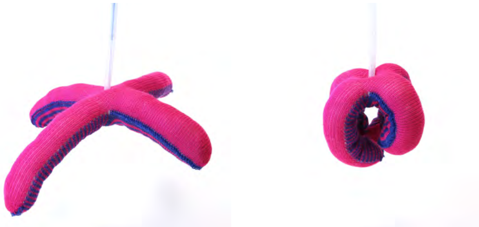
Figure 5.19 The gripper combines both tube types and both tendon types: a horizontal (inlaid) tendon is set into a horizontally-formed tube, and a vertical (yarn tangling) tendon is set into a vertically-formed tube. An eyelet at the intersection of the tendons makes it easy to pull the strings through to a Bowden tube. The gripper is stuffed with cluster stuffing.
