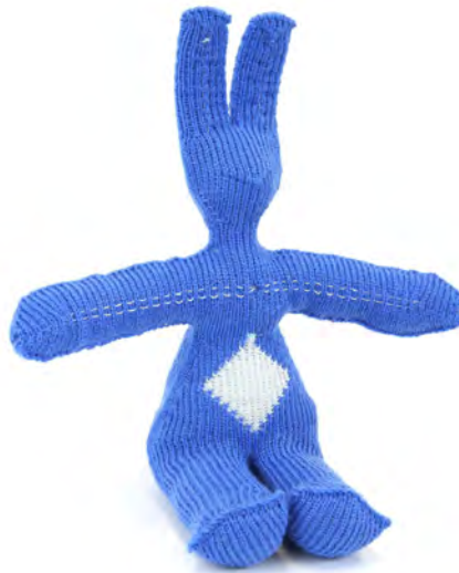
Figure 5.20 The bunny combines both tube types, both tendon types, both shaping techniques, and sensing. It is formed similarly to the gripper, but shows off the shaping complexity that is achievable with short row and increase/decrease shaping. Vertical tendons can actuate the ears, which are stuffed with craft foam. The rest of the bunny is stuffed with cluster stuffing, and horizontal tendons can actuate the arms in a hugging motion. The bunny is primarily knit in Yeoman Yarns “Volga” wool/polyester blend yarn, with an inlay of conductive yarn (Bekaert VN35X4) knit using the “plating” technique with Tamm Petit yarn for strength. a) Schematic of the bunny (not to scale). A: direction of knitting. B: Short rows bend the legs and torso. C: Decreases to shape the torso. D: Short rows at the edges of a horizontal tube provide roundness. E: Increases to shape the neck and head. F: Horizontal tendon for arms. G: Vertical tendons for ears. b) and c) A bunny with conductive belly and separately actuated ears and arms.
