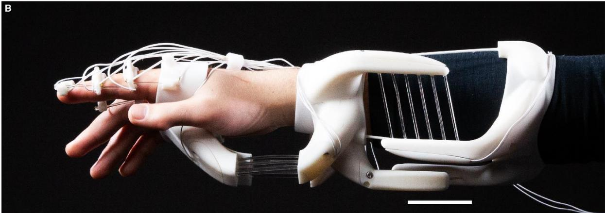
Figure 6-23. The arm-wearable device design. (A) A render of the device design without mechanical features. (B) The final, assembled device. Scale bar, 50 mm.
