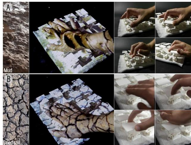
**Figure 5-13. Interacting with the kinematic material display - the display simulating (A) mud with four DOF and (B) stiff dried soil with 2 DOF.**
