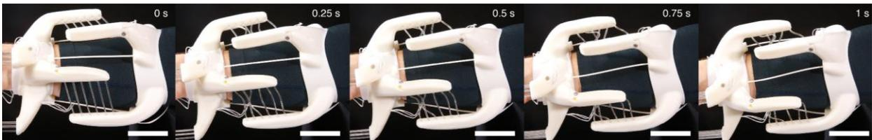
Figure 6-24. Pictures of the arm-wearable device's forearm joint in the unlocked state. Scale bar, 50 mm.
