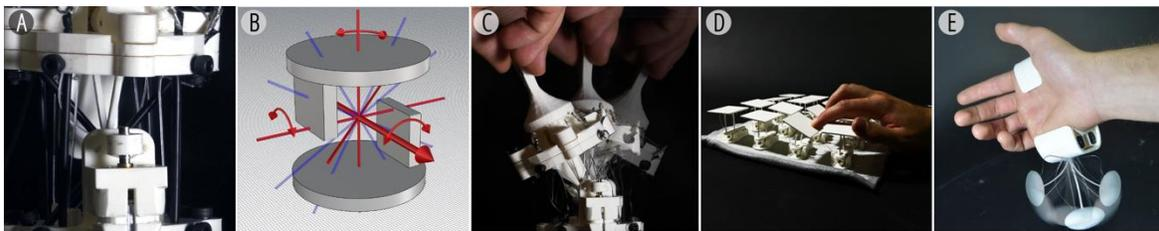
**Figure 5-1. ReCompFig overview - (A) compliant mechanisms that have multiple cable-based reconfigurable kinematic degrees of freedom. (B) Design tool prototype and algorithms based on the screw theory are provided to assist users. Application examples including (C) a multimodal input device, (D) a kinematic material display, and (E) a haptic proxy are provided to demonstrate the enabled interaction design space.**
