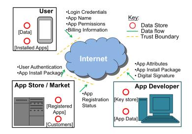
Figure 3.1: The Data Flow Diagram Artifact
